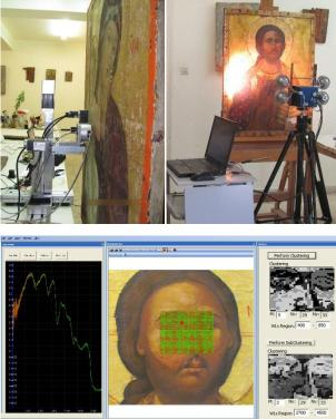
The icon was scanned in situ in the conservation laboratory of the Holy Archbishopric of Cyprus using the prototype spectroscopic and the InSb 640x512 FPA XENICS imaging devices.
